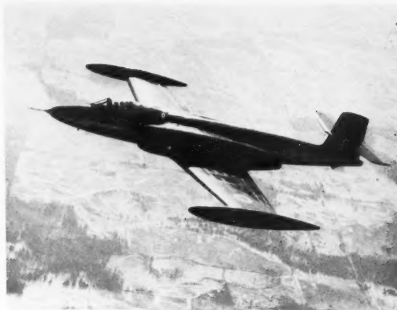
FIG. 3. Avro all-weather fighter (CF-100) in production for the R.C.A.F. at Toronto. Powered by two Avro Orenda engines.
